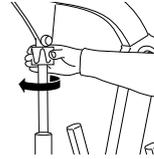
Manually turn the red actuator collar in the direction of the arrows to lower.
